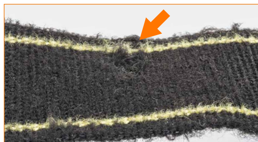
Strap with obvious loose threads.
