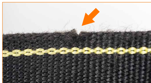
Strap with small tear on external edge.
