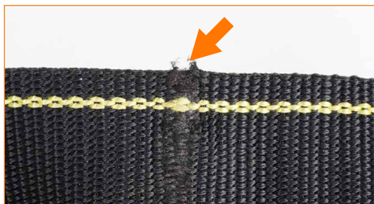
Strap has been crushed.
