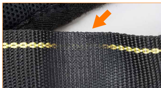
Strap with signs of burning from being near to heat source.
