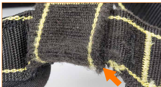
Straps very worn where they join.
