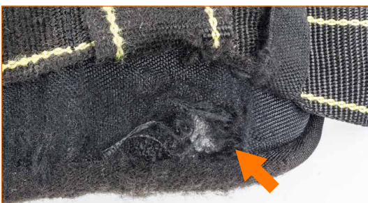
Padding very worn. Wear of non-structural components should not be underestimated because it indicates general wear of the device.
