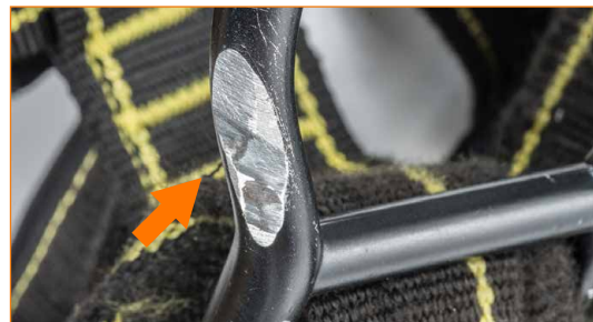
Attachment ring with clear signs of abrasion.
